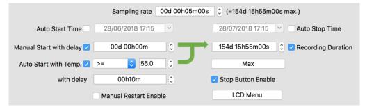
In this example, the logger will start manually by pressing the start button without any delay, or will start automatically if the temperature is greater or equal to 55°C for 10 minutes consecutive. The sampling rate is 5 minutes and the logger will stop automatically after 154 days, 15 hours and 55 minutes.
