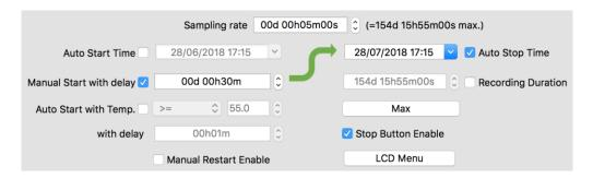
In this example, the logger will start manually by pressing the start button with a delay of 30 minutes. The sampling rate is 5 minutes and the logger will stop automatically at 17H15 on June 28, 2018.
