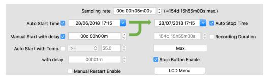
In this example, the logger will start automatically at 17H15 on June 28<sup>th</sup> 2018. It can also be started manually by pressing the start button without any delay. The sampling rate is 5 minutes and the logger will stop automatically at 17H15 on July 28, 2018.
