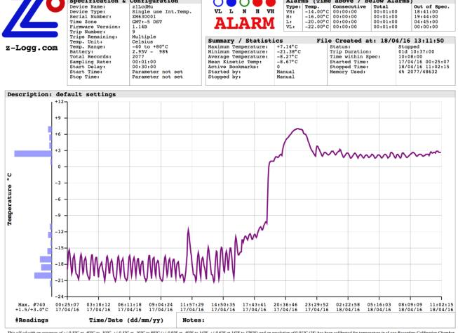
This z1Lcd with an accuracy of +/-0.5°C at -40°C to -10°C, +/-0.3°C at -10°C to 80°C (+/-0.9°F at -40°F to 14°F, +/-0.6°F at 14°F to 176°F) and an resolution of 0.01°C (°F) has been calibrated for temperature in zLogg Recorders Calibration Chamber. The reference equipment used is traceable to National Institute of Standards and Technology. Device:#ZM630001
