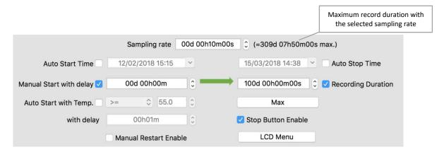
In this example, the logger will start manually by pressing the start button without any delay. The sampling rate is 10 minutes and the logger will stop automatically after 100 days.
