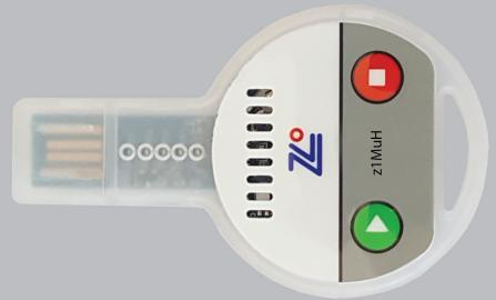
Once plugged into the USB port, the logger works like a USB stick that holds the automatically generated ZLG, TXT, CSV and PDF files. No zLogg software needed.
